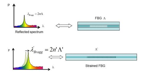
In a case, that an FBG is subject to thermal and mechanical variations at the same time, there is no technique how to distinguish them from each other. To solve this, there are several methods. One possibility is to fabricate a sensor, which is sensitive only to temperature changes. By the means of this temperature sensor it's possible to compensate the temperature effects of a strain sensor.
