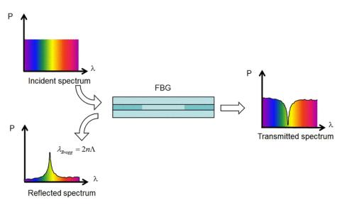
This equation indicates that the Bragg wavelength can be affected by the change of the 2 parameters mentioned above (effective refractive index and grating period). This explains why an FBG is sensitive to strain change and temperature:
