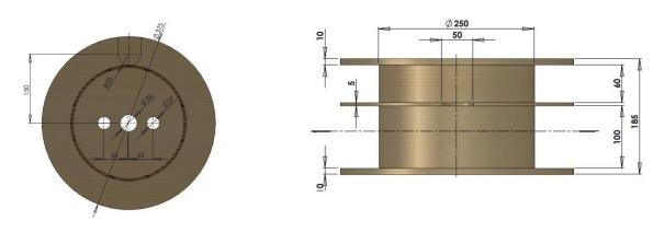
The new reel (POP-UP I) has slightly different dimensions in comparison to the SIZE 0 reel, leading to a higher cable coiling capacity. The new dimensions are shown in the diagrams below:
